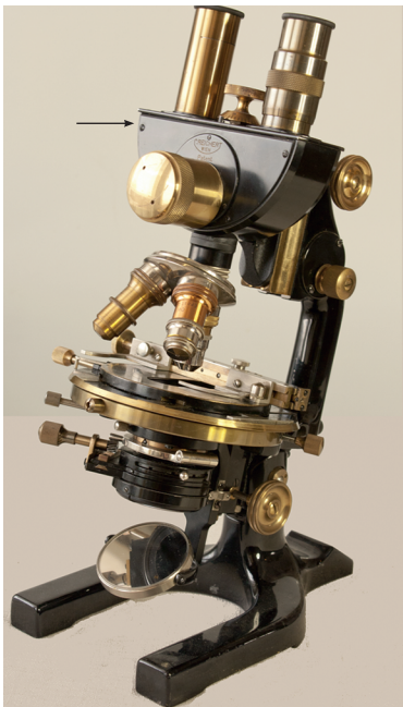
Fig. 2.4. Reichert microscope (Austria) with binocular head (arrow)
